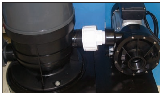
Figure 13b — Side mount pump attached directly the filter tank
