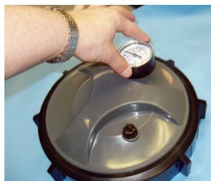
Figure 25b — Installing pressure gauge
