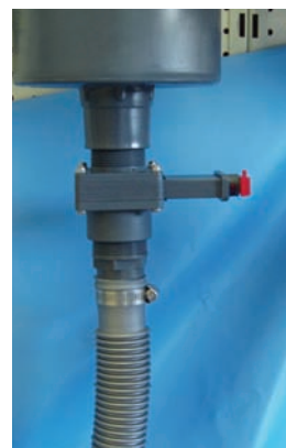
Figure 24 — Slide valve in closed position
